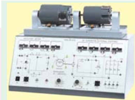
Repulsion induction motor
