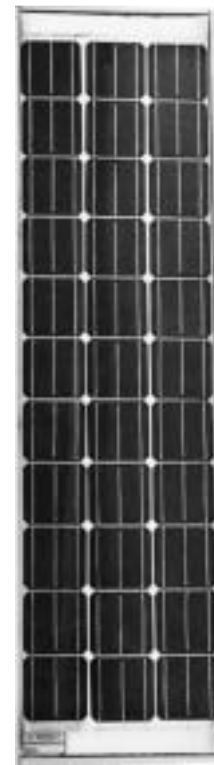
40-W, high-density solar module 100-mm \times 100-mm ( 4'' \times 4'' ) square cells are used to provide maximum power in a minimum of space. The 33 series cell module provides a strong 12-V battery charging current for a wide range of temperatures ( -40^\circ\text{C} to 60^\circ\text{C} )
