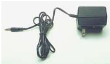
FIG. 2.32 Answering machine/phone 9-V dc supply.
