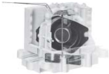
FIG. 13.65 Electrodynamometer movement. (Courtesy of Weston Instruments, Inc.)
