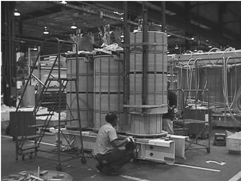
FIGURE 2.1.8 Concentric arrangement, outer coil being lowered onto core leg over top of inner coil.
