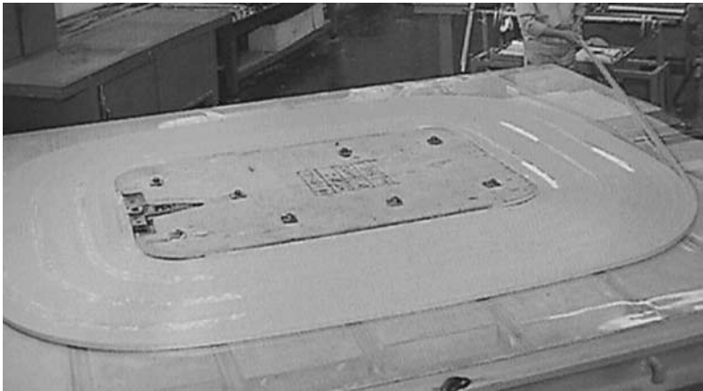
FIGURE 2.1.12 Pancake winding during winding process.
