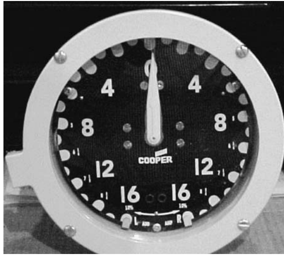
FIGURE 2.7.15 Tap-changer position indicator.
