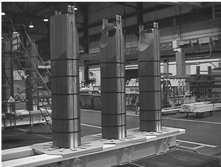
FIGURE 2.1.5 “E”-assembly, prior to addition of coils and insertion of top yoke.
