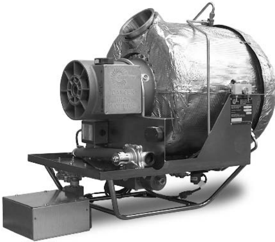
Figure 11-1. Courtesy of Capstone Turbine Corporation. The C30 & C60 microturbine systems are ultra-low-emission combined heat and power generator sets providing up to 30 kW and 60 kW of power, 85 kW and 150 kW of heat, at heat rates of 13,100 Btu/kW-Hr and 12,200 Btu/kW-Hr, respectively.
