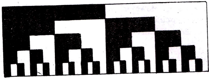
Fig. 25.30. 5-digit scale for digital indication of linear position of a movable object.
