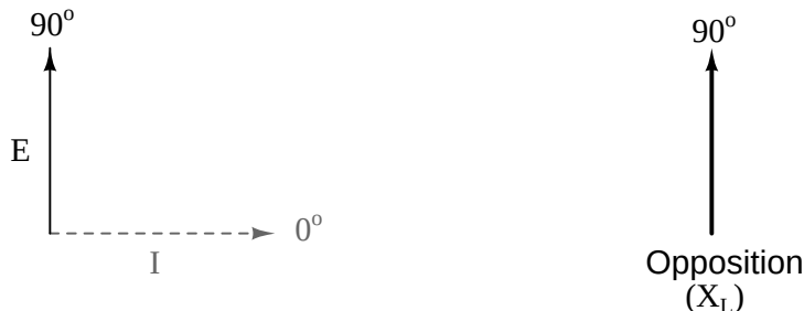
Figure 3.9: Current lags voltage by 90^\circ in an inductor.
