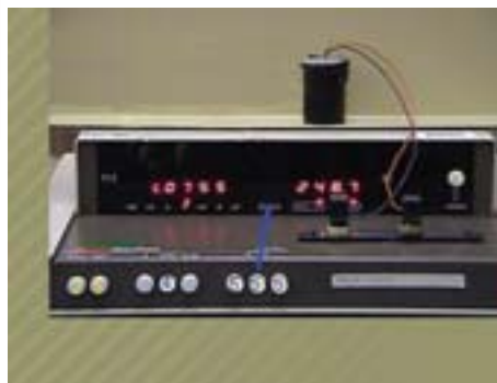
Inductance Measurement using bridge
