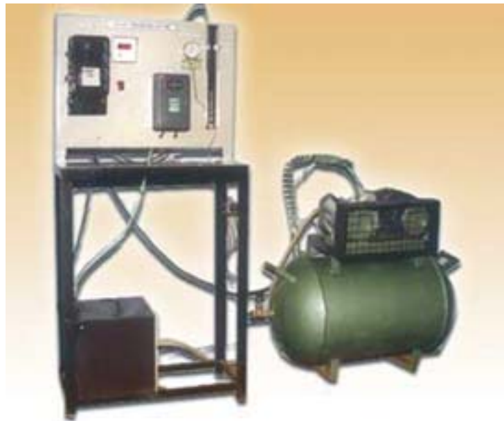
Measuring efficiency of compressor.
