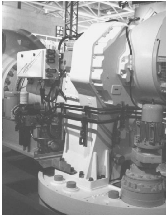
Figure 6.21 Integrated Gearbox on the Zond Z-750 turbine. (The gearbox is mounted on a circular nacelle bedplate, with the hub to the left and generator at the rear. An electrically driven yaw drive can be seen beneath the generator).
