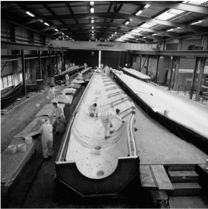
Figure 7.7 Blade Production. View of Veneer Lay-up in Mould to Make One Blade Skin. The Blade is Completed by Glueing Face and Camber Skins Together. (Reproduced by permission of NEG-Micon)
