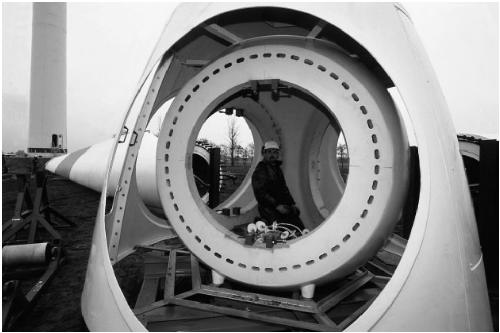
Figure 7.23 Rotor Hub. View of Spherical-shaped Rotor Hub for the 1.5 MW NEG Micon Turbine Awaiting Installation. The Hub and Spinner are Temporarily Oriented with the Rotor Shaft Axis Vertical. The Turbine is Stall-regulated, so Slotted Blade Fixing Holes are Provided to Allow for Fine Adjustment of Blade Pitch to Suit the Site. (Reproduced by permission of NEG-Micon)
