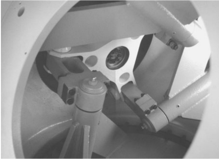
Figure 6.8 Pitch Linkage System Used in Conjunction with a Single Hydraulic Actuator Located in the Nacelle. (The central triangular 'spider' is connected to the actuator by a rod passing through the hollow low-speed shaft. Links from the spider drive the blade pitch via braced arms cantilevering into the hub from each blade. Each arm is parallel to its blade axis, but eccentric to it).
