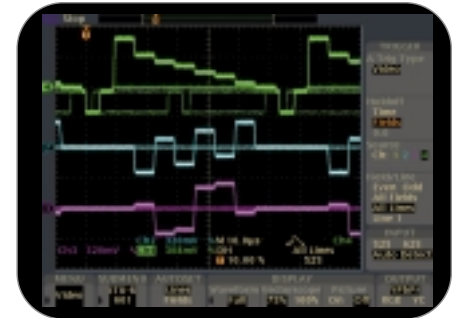
► Figure 58. The TDS3SDI video module makes the TDS3000 Series oscilloscope a fast, tell-all tool for video troubleshooting.
