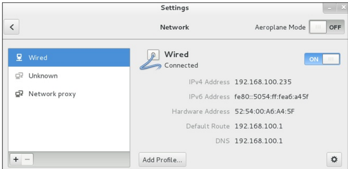
Figure 2.3. Configure Networks Using the Network Settings Window
